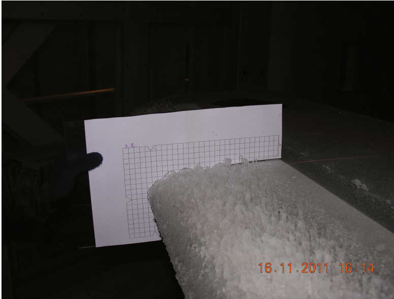
Figure 7.3: Photograph of the traced ice shape on the tip section of the Dassault wing, picture from CIRA
